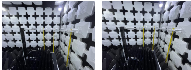
Figure 6. Photos of OTA test in EMC anechoic chamber of test sample
